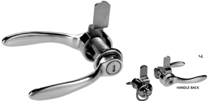
43.1029 Cam latch with levers and key lock. For up to 1 inch or 25 mm door thickness. Cam action: 2 inches max. (see different cams) Lever and cam have a 180 degree swing when unlocked. Lever is 3 1/2 inch long; comes with 3 installation options:
