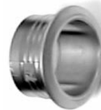
Plastic Ring for 3/4" thick material; drill hole 26 mm diameter
