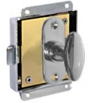
Latch #21.709-30; 30 mm backset, brass chrome plated 7 x 7 mm spindle SET: 21.719-30 #16.087 oval knob with #oval rose
